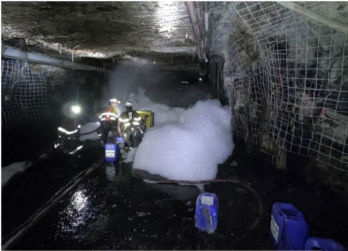
Figure 5 Photo shown to firefighting responders at incident site using Turbex foam generator
