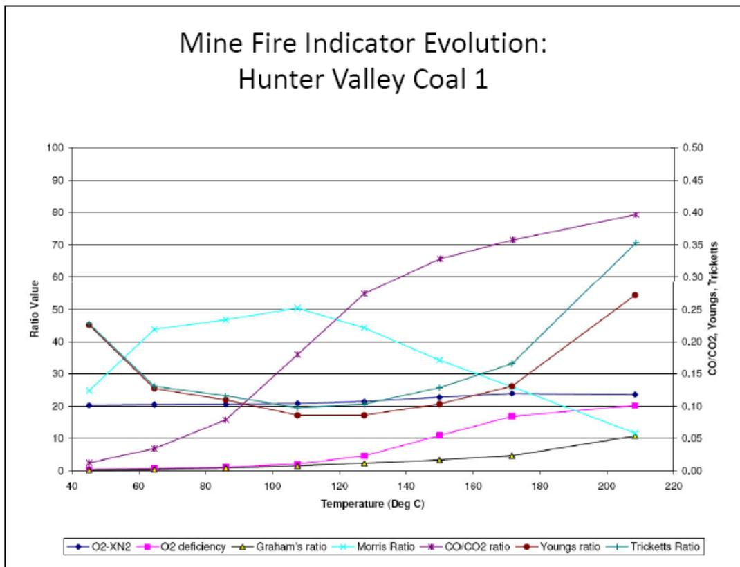
When the results of a number of analyses of atmospheric samples from heating sites are plotted there will inevitably be a number of readings which appear to be anomalous. There is also likely to be a somewhat irregular progression from one sample result to another. This occurs because:
