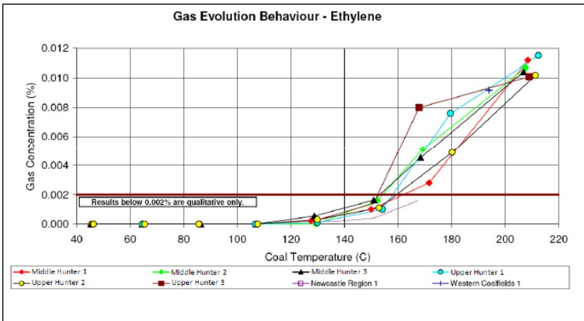
Indicators of spontaneous combustion risk should include both gas analysis based and other sensory or observation based indicators. Heatings can only be detected in the early stage if monitoring takes place in or near where heatings can occur.
