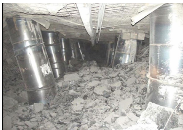
Figure 32. Elk Creek longwall tailgate coalburst (Mark 2016)
