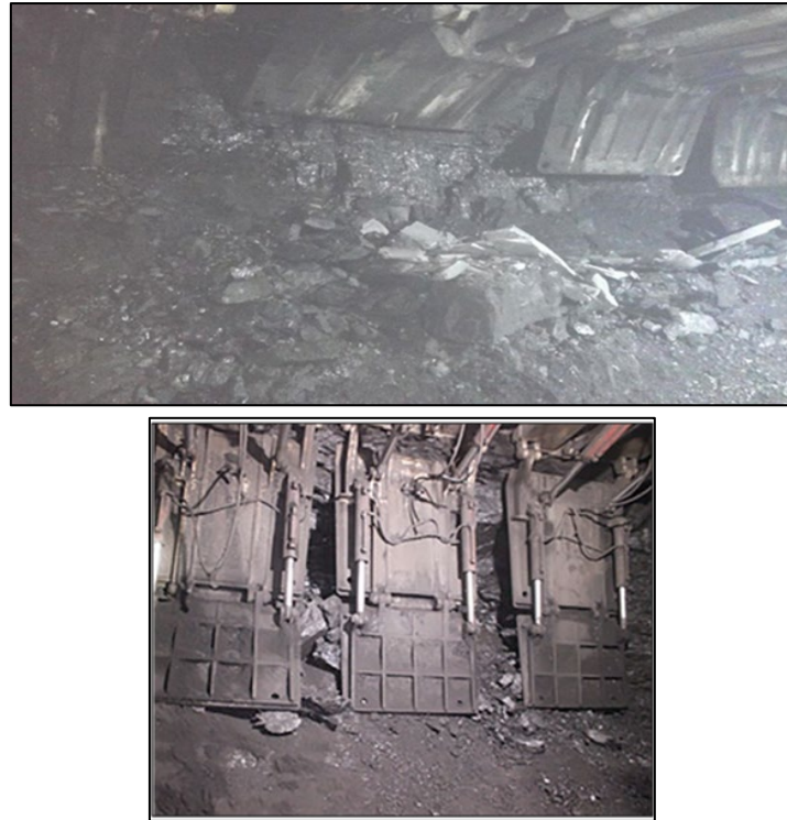
Figure 34. Shangwan rib spall on a longwall face (Zhang, 2016) and hard coal thick seam longwall face (Wang, 2018b)
