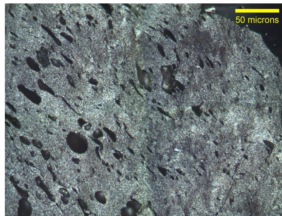
Figure 22. Microscopic structure of heat-affected coal displaying mosaic structure (Beamish, 2016)
