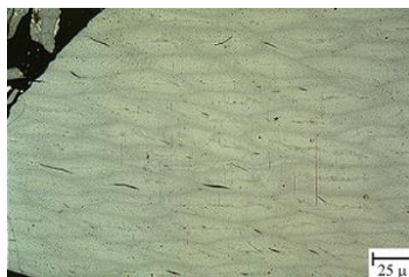
Figure 23. Microscopic structure of naturally rank advanced coal (Southern Illinois University, 2016)
