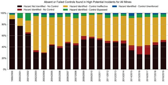
Figure 38 Absent/Failed defences for HPIs over time (normalised)
