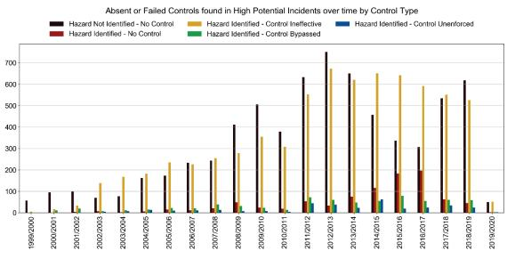
Figure 37 Absent/Failed defences for HPIs over time
