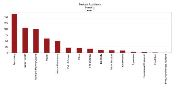
Figure 4 shows the hazards for Serious Accidents.
